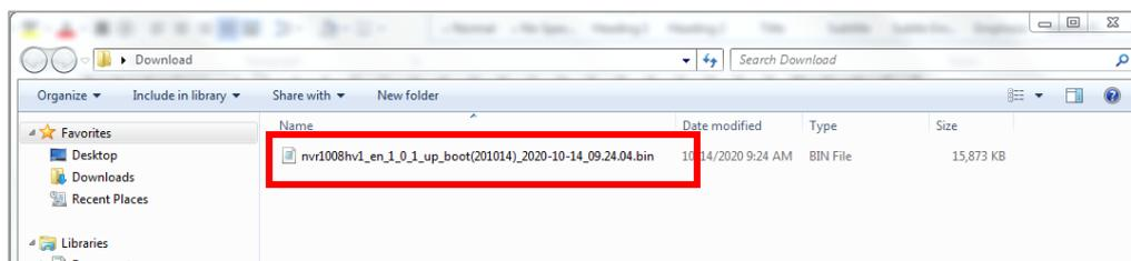
1.3 To upgrade the firmware via VIGI NVR locally, please get a USB drive and copy the .bin file to it. Then plug this drive to the USB port of VIGI NVR for the [next step](#).
