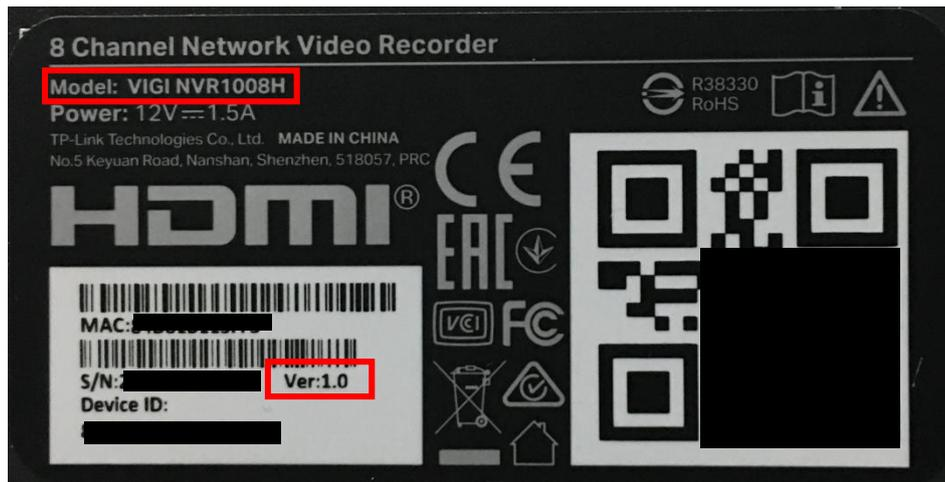
1.2 Download the corresponding firmware according to the VIGI NVR's model and hardware version from TP-Link official website <https://www.tp-link.com/support/>. Then extract the file and get the .bin file for the upgrade.
